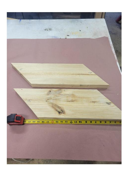
On the bottom of the long legs measure 6" up from the short point and mark the spot. Measure 13" up from the long point and mark the spot. Connect the dots with a straight edge. The line should be at a slight angle. This will be the guide line to where the short leg will be attached to the long leg. See photo below.
