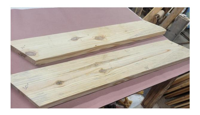
On one end of the long legs measure 17 ½" down from the point and mark the spot. Then measure 4" over from the short point and connect the dots. The shaded area will be cut off leaving the back taper for the seat back. Repeat this step on the other long leg so that you have to pieces with a taper. See photo below.
