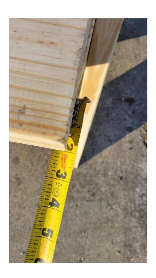
Now attach the two 48" back slats. The top board may overhang the top by ½" due to the angle. Use four 3" deck screws and screw the top board in place. Two screws on each side. The bottom board will sit flush with the bottom taper of the long leg. Use four 3" deck screws to attach. Two screws on each side. See photo below.
